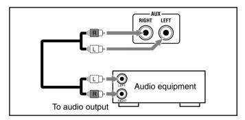
For playing the other equipment through this unit, connect between the audio output jacks on the other equipment and AUX jacks by using an audio cord (not supplied).
